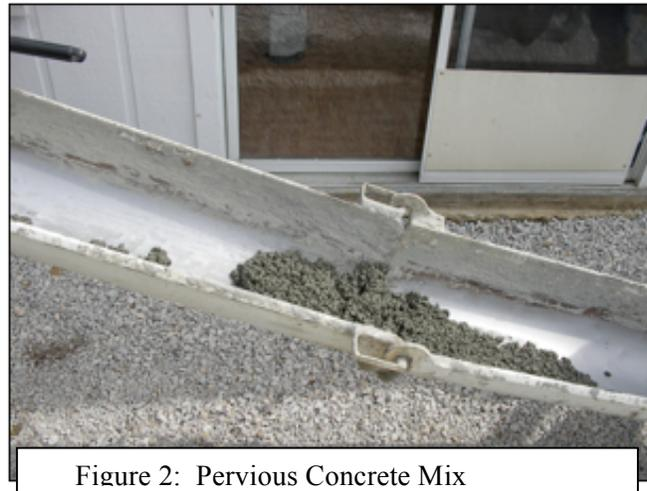
Figure 2: Pervious Concrete Mix
